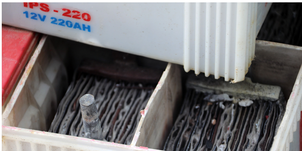
← Image 1. Lead-containing waste generated at an informal LAB breaking site. Limited traceability in informal recycling activities affects the monitoring of hazardous materials and the verification of environmentally sound waste management practices.
