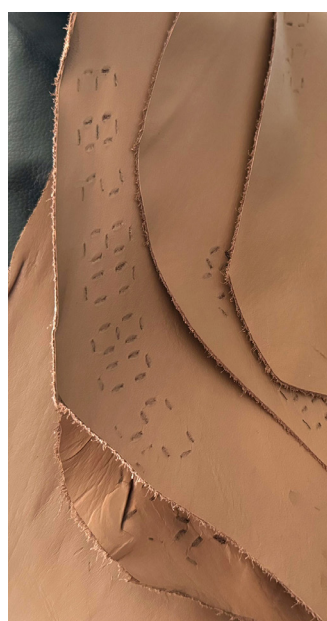
↑ Image 17. Finished leather hides marked with engraved identification codes that enable traceability throughout the leather value chain in a SMEP-supported pilot in Pakistan.
