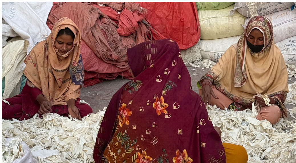
← Image 2. Workers sorting textile production off-cuts. Capturing information on material origin and fibre composition at this stage increases traceability and supports chain-of-custody verification in downstream textile-to-textile recycling.
