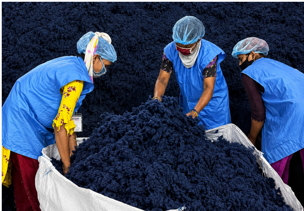
← Image 18. Handling coloured textile fibres during processing. Fibre blending and processing stages are critical traceability hotspots, where information on fibre composition and chemical inputs may be lost.
